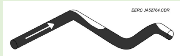
Illustration of slack pipeline flow
